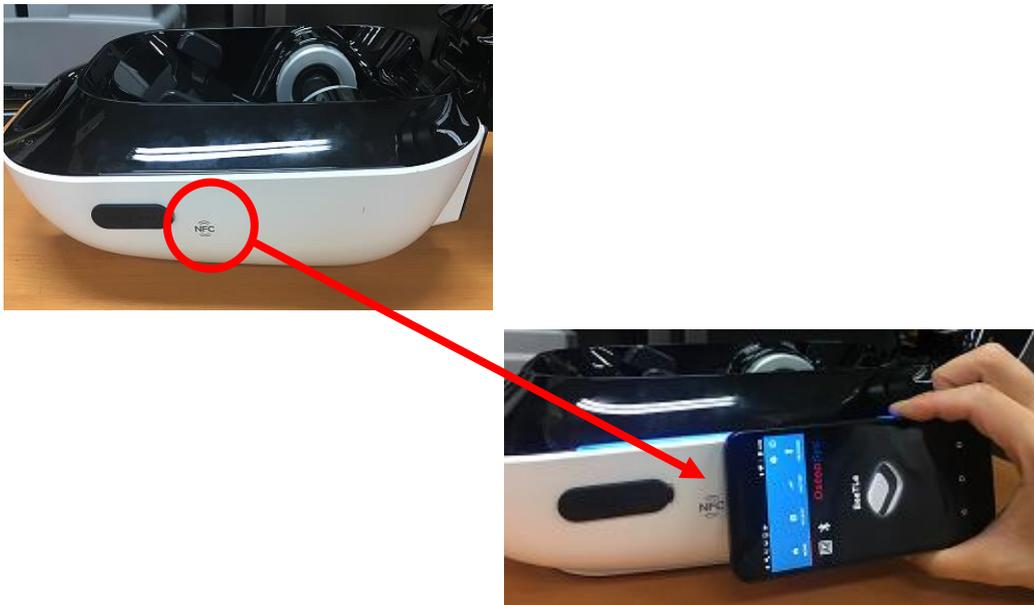
(1) Place your smart device near the NFC mark on the BeeTLe
