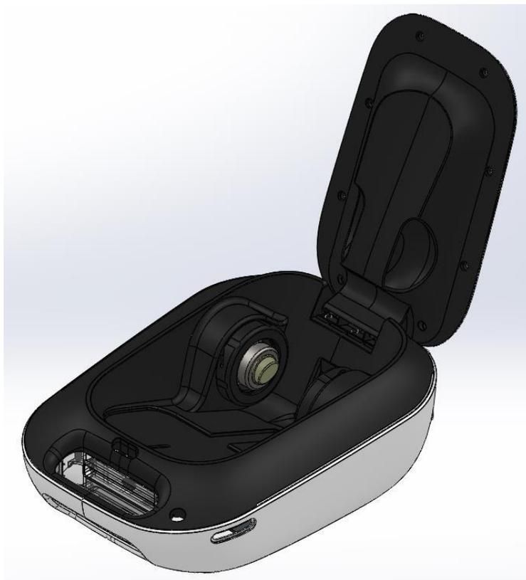
BeeTLe is a bone densitometry device to measure and prevent osteoporosis by measuring the bone mineral density of Calcaneus using ultrasound.
