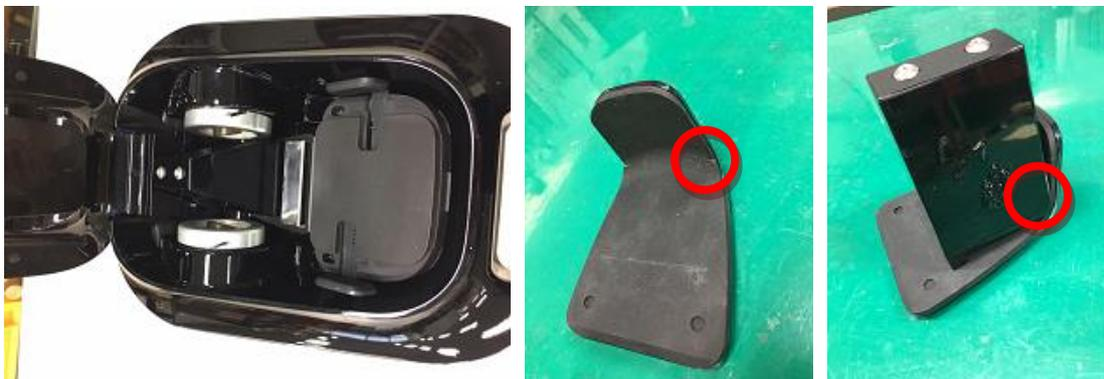
Start Daily test, lightly push down the foot supporter as shown in the picture below.
